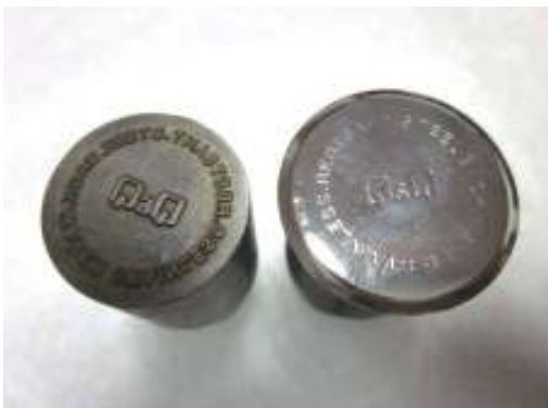
Counterfeit "Q&Q" watch back case production mould
